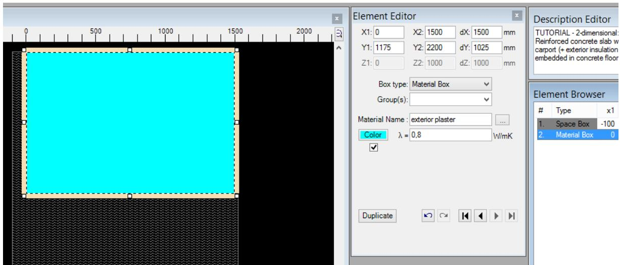
This time enter “Material box” as the “Element Type“. In the field “Material name” enter “plaster”. “Lambda” should be assigned a value of “0.8”.
