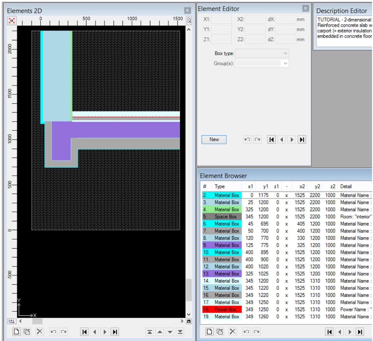
For the first significant results (building component properties and U values) and to check the input go to: **View** → **Evaluation&Reports** → **Modelling Report**
